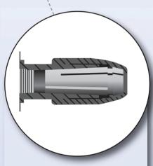
The all new design of the SMD's clamping system, which incorporates a collet and cap-nut assembly, ensures that the consumable is exceptionally securely located within the chuck. Additionally, the design and operation of the clamping system produces highly consistent run out.
